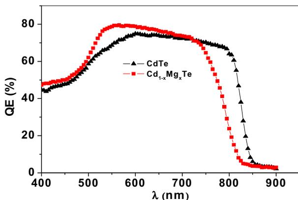
Fig. 1. Quantum efficiency spectra of  $\text{Cd}_{1-x}\text{Mg}_x\text{Te}/\text{CdS}$  and CdTe/CdS devices.
