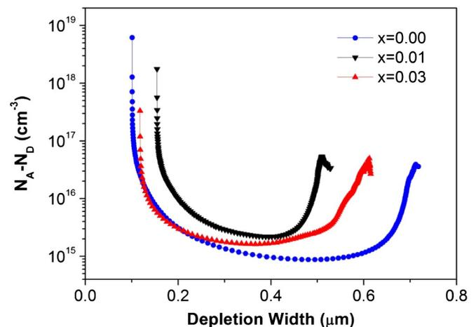
Fig. 3. Capacitance depth profiles for  $\text{Cd}_{1-x}\text{Mg}_x\text{Te}/\text{CdS}$  devices ( $x = 0.00, 0.01$  and  $0.03$ ).
