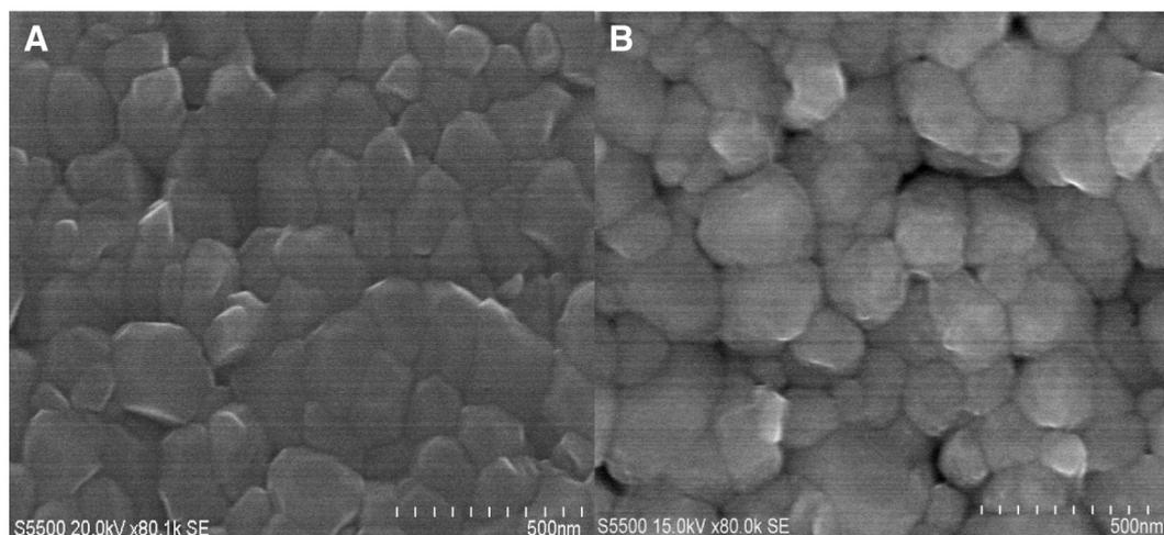
**Fig. 5.** SEM images of  $\text{Cd}_{1-x}\text{Mg}_x\text{Te}$  films: A—annealed without  $\text{CdCl}_2$ , B—annealed in presence of  $\text{CdCl}_2$ . Annealing temperature was 400 °C for 5 min.
