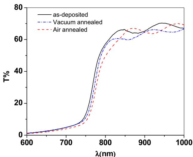
**Fig. 4.** Transmittance spectra of  $\text{Cd}_{1-x}\text{Mg}_x\text{Te}$  Films: as-deposited, annealed with  $\text{CdCl}_2$  in vacuum, and annealed with  $\text{CdCl}_2$  in air.
