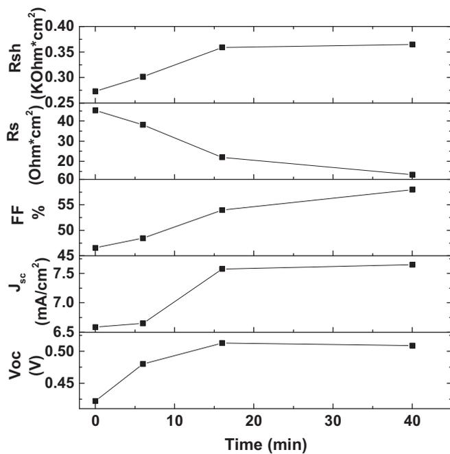
Fig. 6. Diffusion time of Cu contact vs. electrical parameters ( $V_{oc}$ ,  $J_{sc}$ , FF,  $R_s$  and  $R_{sh}$ ) of a typical  $Cd_{1-x}Mg_xTe/CdS$  device. Cu/Au = 3 nm/30 nm, temperature of diffusion 150 °C.
